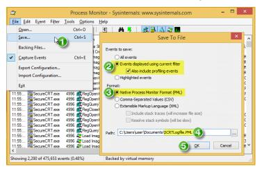
10) Compress the .PML file that was generated (zip) and send it as an email attachment to the technical support representative with which you have been corresponding at VanDyke Software.
